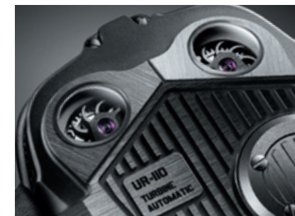
In the UR-110, two turbines are geared to the rotor, which engages the winding system in only one direction of spin. These turbines are not adjustable, but their curved blades offer increased air resistance to the rotor's free direction of spin, and less resistance to its winding rotation, thereby encouraging the rotor to do its duty.
