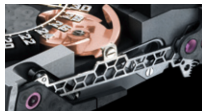
The pink cam lifts and drops the honeycomb arm. The rack at its far end rotates the cylinders for the linear minutes and hours.
