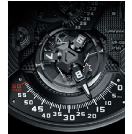
In the UR-1001 time device, the minutes pointer leaves its satellite hour at the end of the hour and slides back to join the next hour at the start of the minutes scale.
