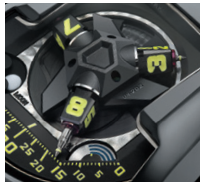
Three transporters push the telescoping hands in and out to follow the vectors of the minutes scale. The groove that the transporters follow can be seen cut into the base of the case on the left.
