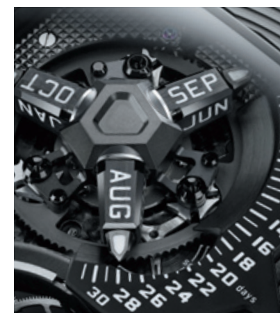
The revolving satellite calendar in the UR-1001 device shows the months, in three groups of four, successively moving across a scale of 31 days on a carousel that advances every 24 hours. The dates are self-adjusting for months of 30 and 31 days but need to be set manually to March 1 on the last day of February.
